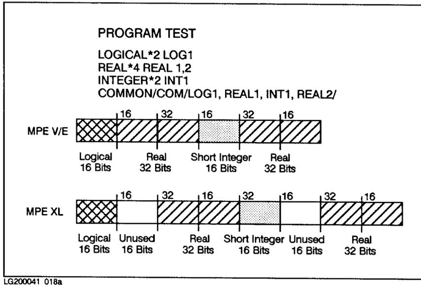
**Figure 10-1. HP FORTRAN 77 COMMON Block Data Alignment Example**
