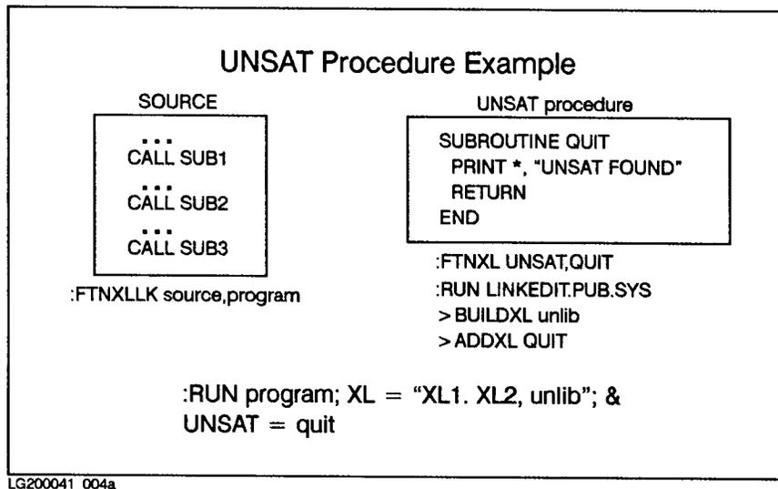
**Figure 2-1. UNSAT Procedure**
